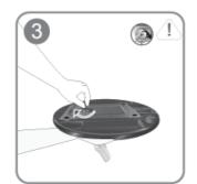
Turn the connecting screw at the bottom of the stand fully so that it is completely fixed.
